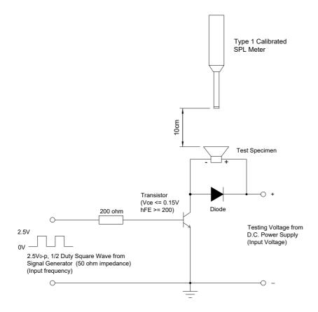
Figure 1. Test Setup
