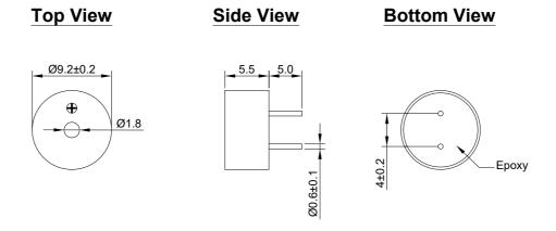
Figure 2. HC0905T/208 Mechanical Layout
